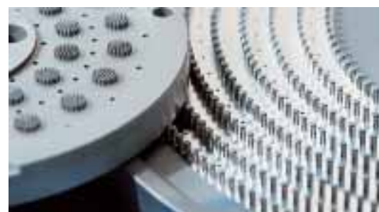
Spinnerets determine the final quality of synthetic yarns.
