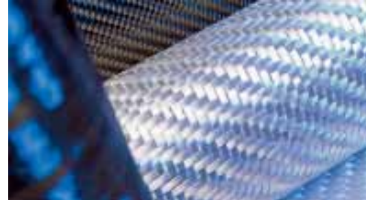
Many composites consist of prepregs: glass, aramid or carbon fibers or fabrics impregnated with specially formulated resins.
